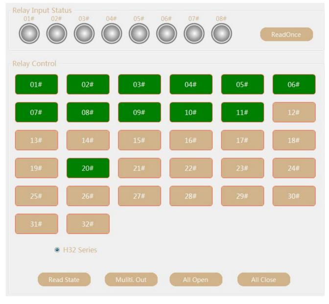
Relay Input Status---01#--08# input port of KC868-Hx controller [ReadOnce]:Read input status of KC868-Hx controller for one time.
