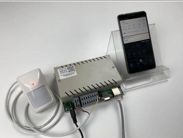
A photograph showing a white human infrared detector connected to a central grey hub. The hub is connected to a smartphone mounted on a clear stand, which displays a monitoring application. Wires connect the detector to the hub, and the hub to the smartphone. |
