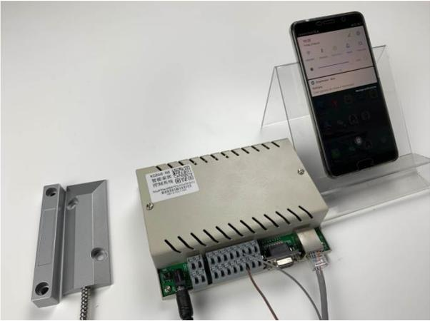
A photograph showing a grey door magnet sensor connected to a central grey hub. The hub is connected to a smartphone mounted on a clear stand, which displays a monitoring application. Wires connect the sensor to the hub, and the hub to the smartphone.          |
