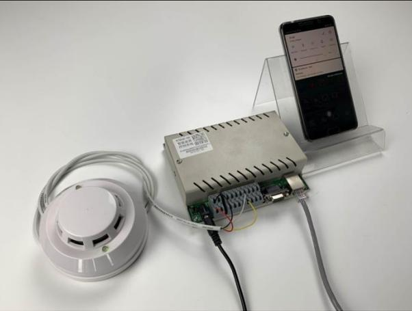
A photograph showing a white gas sensor connected to a central grey hub. The hub is connected to a smartphone mounted on a clear stand, which displays a monitoring application. Wires connect the sensor to the hub, and the hub to the smartphone.               |
