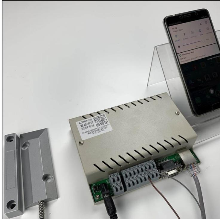
**Door Magnet Sensor connects to the Device (Brown and Grey wires)
