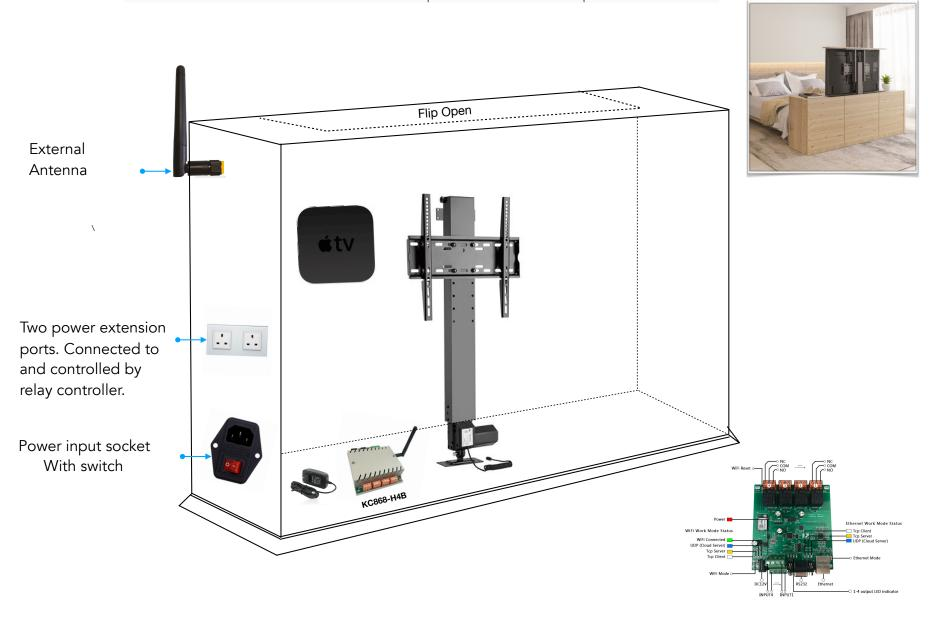
Note: KC868-H4B can be integrated (Ethernet / WiFi) with Loxone using virtual outputs. The motor can be controlled (TV lift up/down) precisely using the "Automation Blinds" function block of Loxone config. Tu - is time in seconds required to fully lift to the max position. Td - is the time in seconds required to fully lower the TV. Any desired position of the lift is also possible through the function block.
