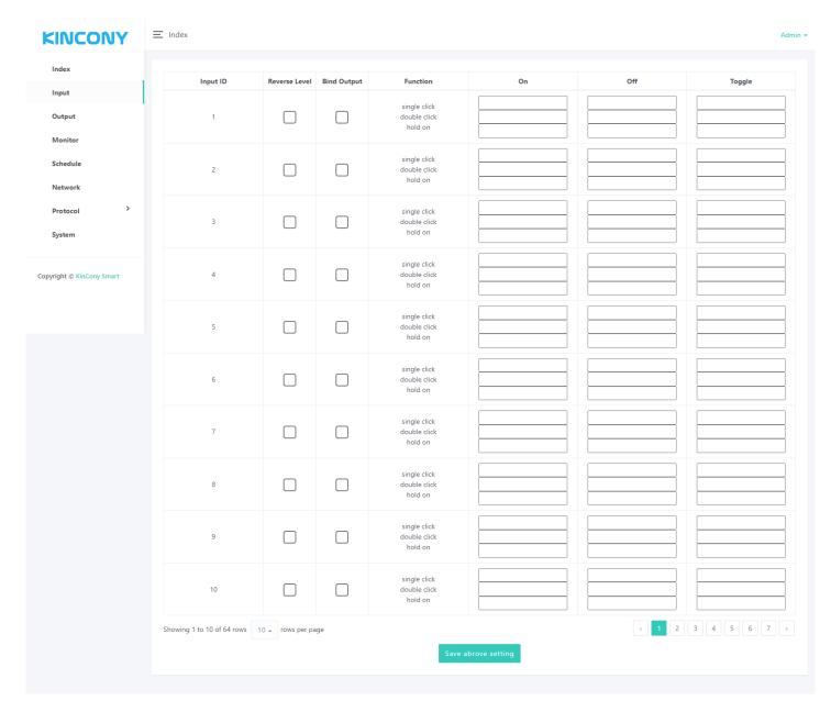
Here is INPUT webpage. Set every digital input port how to work with OUTPUT ports.
