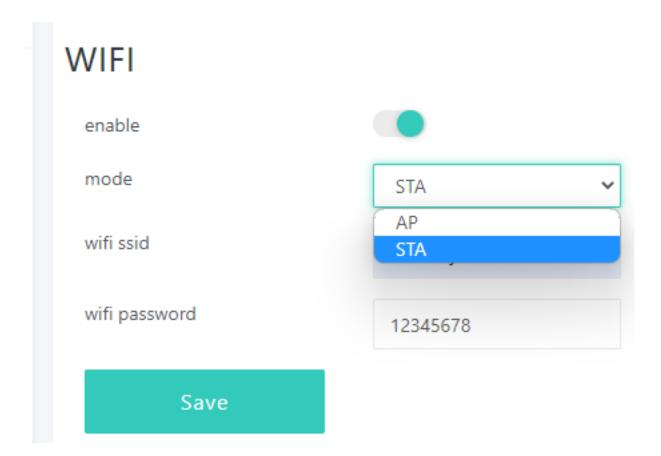
If you set WiFi to STA mode, also you have connect to router by ethernet cable. Board will use ethernet firstly, if ethernet cable disconnected, then will auto switch to WiFi connect to your wifi router, so that make sure let board always connect to your router.
