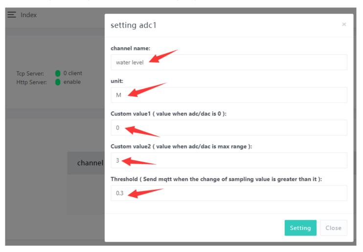
Fox example, we set a water level analog sensor, name is "water level", unit is M (meter), Custom value1 and value2 means: if you are using DC 0-5v analog sensor, when sensor voltage is 0v, what's "Custom value1" corresponding value. when sensor
