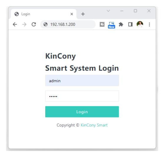
You can login webpage by ethernet IP or WiFi IP. Here is sample login by ethernet IP address 192.168.1.200
